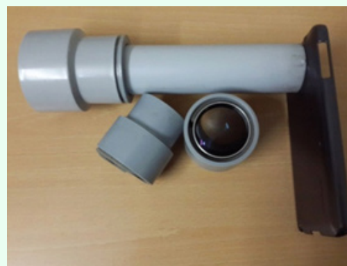
Figure 3: DIY adaptors using PVC pipes (Courtesy: John Davis Akkara)
